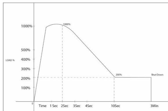
Torque Load Handling Curve
